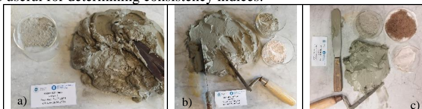
Figure 2. Sample preparation for Consistency Index determination.
